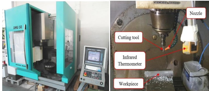
Figure1: Deckel Maho DMU 50 milling machine and the experimental Setup
